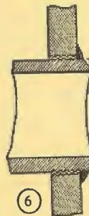
INCORRECTLY WELDED STAY TUBE
